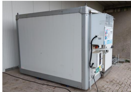
Fig. 2 Climate container for storage of beet sample bags at 9 °C.
