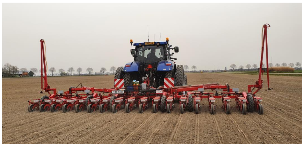
Figure 1. Row fertilization was done in one pass during seeding. In 2022, the coulter furrow was not properly covered with soil. As no rain fell 14 days after sowing, volatilisation of ammonia was possible.
