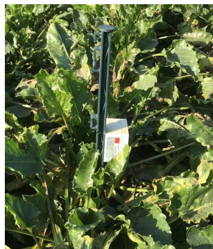
Figure 1. LoRa sensor for temperature and relative humidity in the sugar beet canopy
